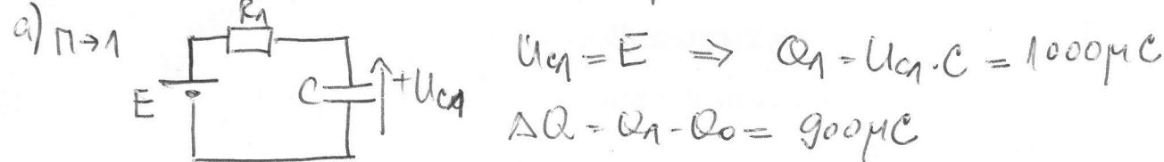
b)  $T_0 = R_1 C \Rightarrow R_1 = \frac{T_0}{C} = \frac{0,05\text{ s}}{100\mu F} = 500\Omega$
