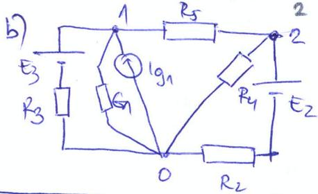
$$\begin{aligned} \left(\frac{1}{R_3} + G_1 + \frac{1}{R_5}\right)U_{10} - \frac{1}{R_5}U_{20} &= \frac{E_3}{R_3} + I_{g1} \\ -\frac{1}{R_5}U_{10} + \left(\frac{1}{R_5} + \frac{1}{R_4} + \frac{1}{R_2}\right)U_{20} &= \frac{E_2}{R_2} \end{aligned}$$
