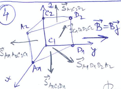
$$\begin{aligned} \Phi_{A_2D_2C_2} &= \vec{B} \cdot \vec{S}_{A_2D_2C_2} = B S_{A_2D_2C_2} \cos \angle(\vec{B}, \vec{S}_{A_2D_2C_2}) \\ &= B S_{A_2D_2C_2} \cos 90^\circ = 0 \end{aligned}$$
