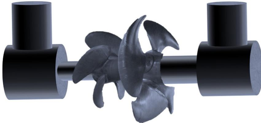
**Fig. 6-14** *Example of a contra-rotating propeller*
