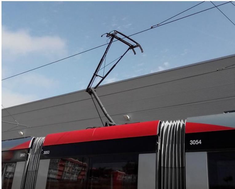
**Fig. 5-11** Pantograph raised on vehicle roof (Source: CAF P&A. Reproduced with permission of CAF P&A)
