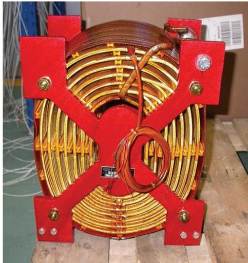
**Fig. 5-16** Air core filter inductor (Source: CAF P&A. Reproduced with permission of CAF P&A)
