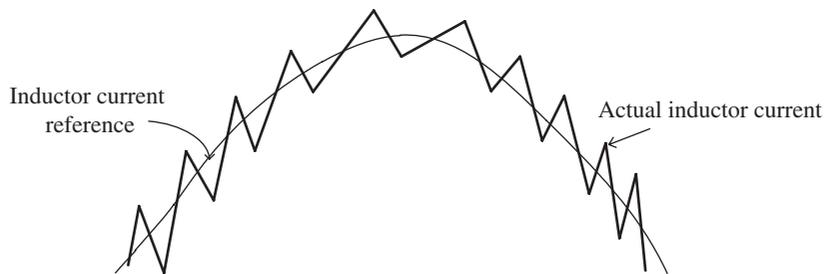
**Fig. 7-60** Typical current mode waveform
