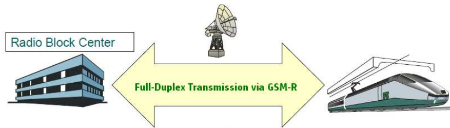
Figure 19: Exchange of information between RBC and trainborne
