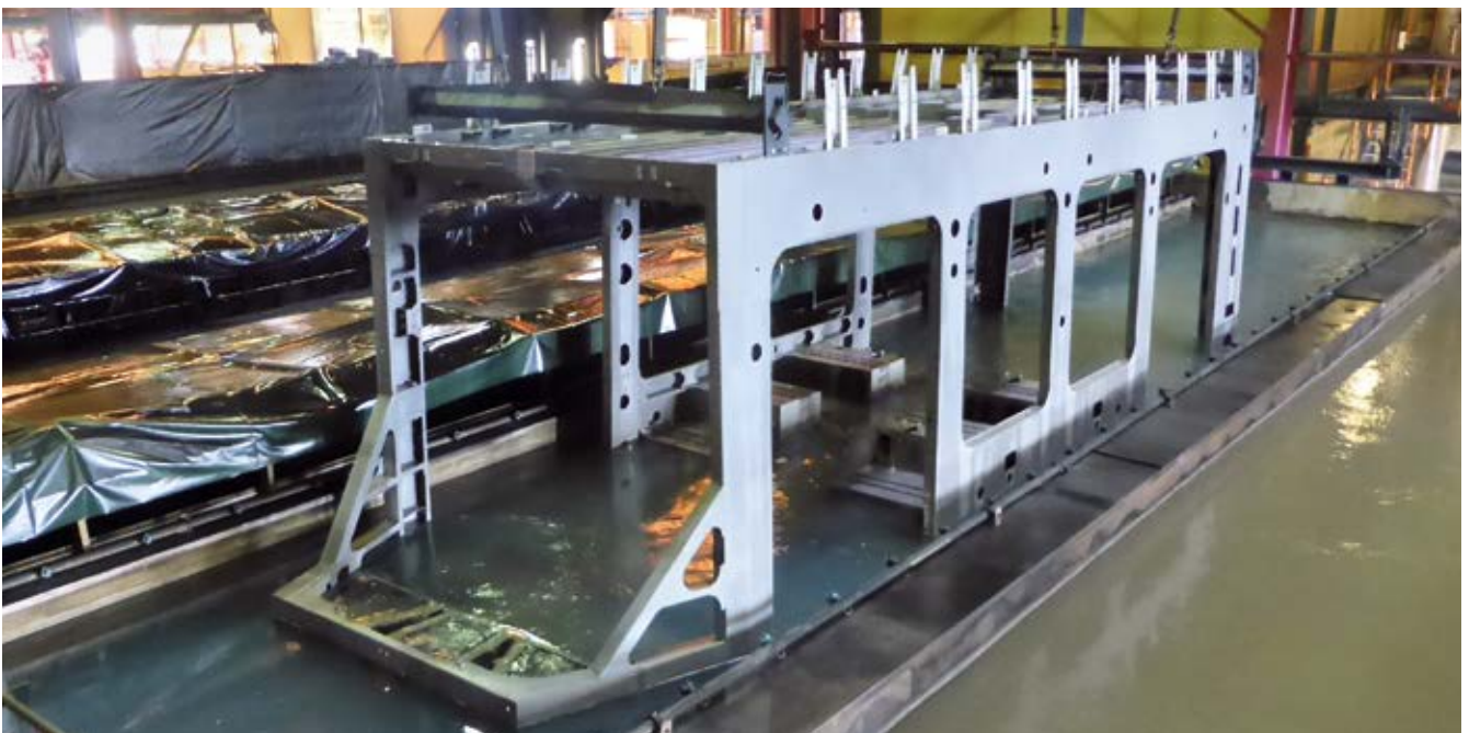
Fig. 5: Avenio carbody during cathodic dip painting
