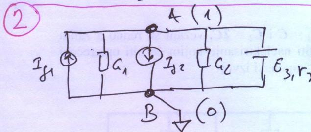
$$P_{I_{g1}} = U_{AB} \cdot I_{g1} = I_{g1}(I_{g1} - I_{g2} + E_3/r_3) / (G_1 + G_2 + 1/r_3)$$
