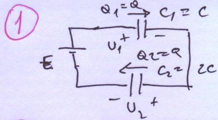
$$C_e = \frac{C_1 C_2}{C_1 + C_2} = \frac{C \cdot 2C}{C + 2C} = \frac{2}{3} C$$
