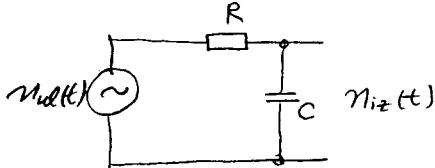
$$H(j\omega) = \frac{X_C}{R + X_C} = \frac{\frac{1}{j\omega C}}{R + \frac{1}{j\omega C}} = \frac{1}{1 + j\omega RC}$$
