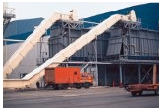
Wood chip handling at 900m 3 per hour
