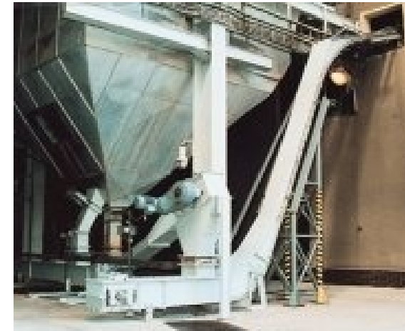
En-masse elevator handling fly ash
